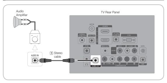
1. Connect the AUDIO OUT port of the TV and the Audio In port of the audio amplifier with a stereo cable.
